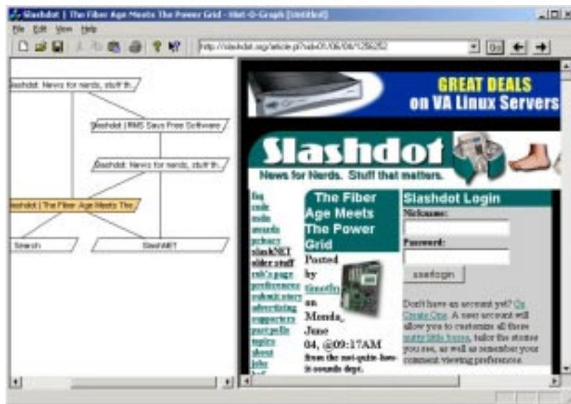
Fig. 1. Histogram screenshot. This application was written as a 100 line C++ program that combines the Dynagraph and Microsoft Internet Explorer COM objects. The graph is a clickable nonlinear history display.
