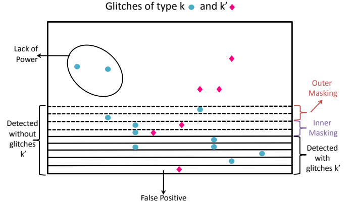
Fig. 1. Inner and outer masking: Glitches of type k (blue dots) that are detectable become undetectable (dashed lines) with the introduction of glitches of type k' (pink diamonds). If k' and k are in the same record i , it is inner masking , and if they are in different records it is outer masking . In addition, a method of detection would also result in false positives (bottom record) and false negatives (shown inside ellipse on top left of the figure).
