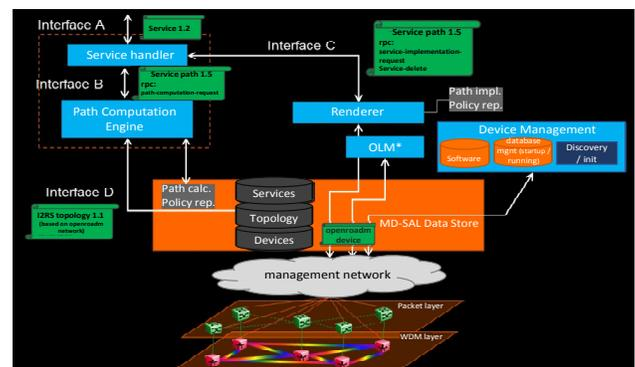
Figure 2: Schematic of Open ROADM Controller Architecture
