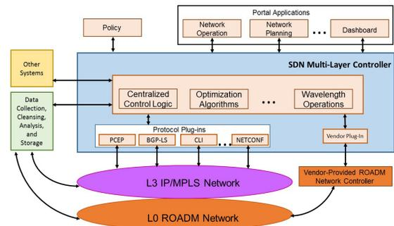
Figure 1: Schematic of SDN Network Architecture
