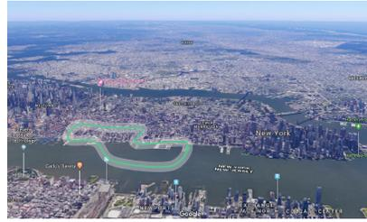
Figure 2: The green line is a planned flight trajectory. The gray buffer defines the flight zone for the aircraft.
